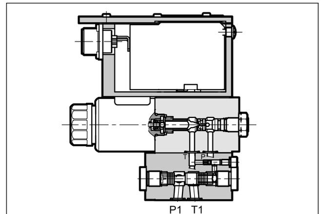
— The PRE3G valve is a pilot operated pressure control valve with electric proportional control and mounting surface in compliance with ISO 4401 standards, controlled by an integral digital amplifier.
