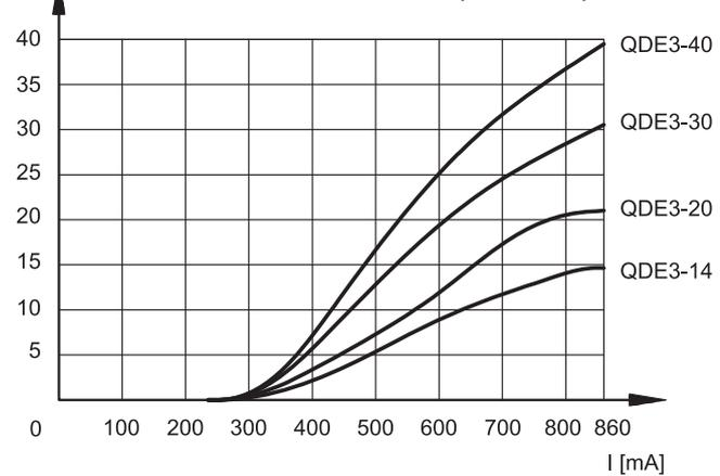
Typical flow rate characteristics A → B for controlled flow rate: 14 - 20 - 30 - 40 l/min in function of the current supplied to the solenoid (D24 version, maximum current 860 mA, PWM 100 Hz)
