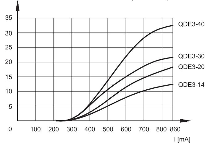
Typical flow rate characteristics A → B for controlled flow rate: 14 - 20 - 30 - 40 l/min in function of the current supplied to the solenoid (D24 version, maximum current 860 mA, PWM 100 Hz)
