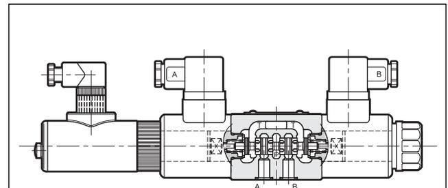
The DSE3F is a direct operated directional valve with proportional control, electrical feedback and mounting interface in compliance with ISO 4401 (CETOP RP 121H) standards.
