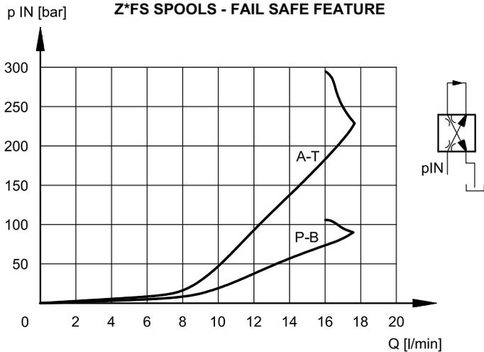
Flow P→B / A→T with valve in fail safe position, depending on the incoming pressure.
