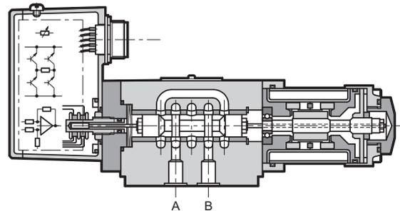
— The DXJ5 is a four-way servo-proportional valve where the spool moves inside a sleeve. This valve has a direct drive with a linear force motor resulting in high dynamic performances independent of system pressure. A linear transducer (LVDT) with closed loop controls the spool position, ensuring high precision and repeatability.
