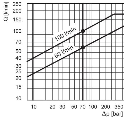
Typical flow rate curves at constant  $\Delta p = 70$  bar P-T according to the reference signal.
