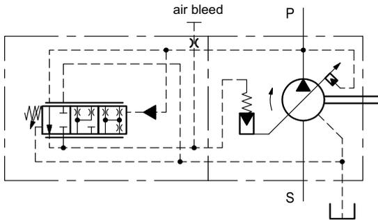
The PC pressure regulator keeps the pressure at a constant set level in the circuit, thus adjusting automatically the pump flow rate according to the real need of the system.
