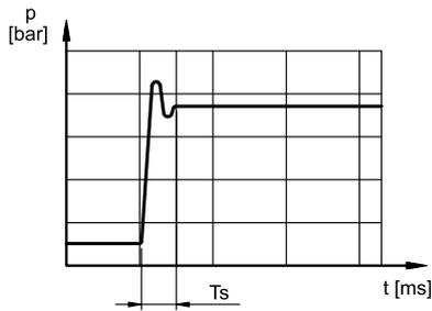
Dynamic response curves obtained by switching the solenoid operated directional valve for closing the pump outlet.
